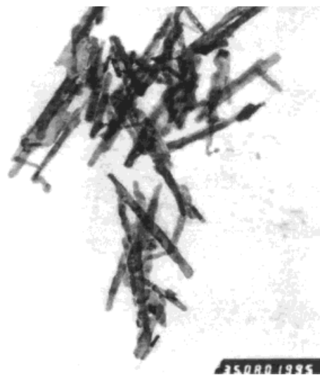
Figure 3 TEM image of copolymer nanofibrils.
